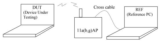
Configuration of equipment for transmitting-receiving test
